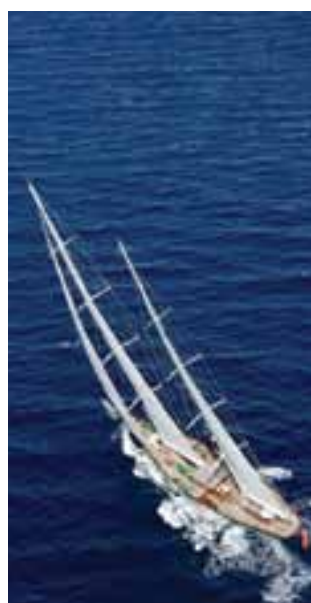
these pages North Sails utilized its new 3Di sail material to meet the owner's demands for performance and technology. 3Di features a composite structure of interleaved spread filament tapes that hold their shape, allowing upwind sails to approach the performance of a rigid foil.
