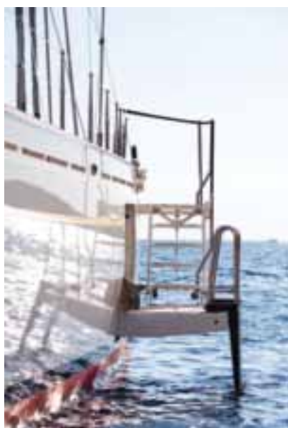
A SIDE-BOARDING PLATFORM IS RECESSED INTO THE HULL AMIDSHIPS TO STARBOARD, ALLOWING FOR EASY ACCESS TO THE SEA FOR SWIMMING & A STABLE AREA FOR TENDERS WITH LESS PITCHING THAN TRANSOM BOARDING.
